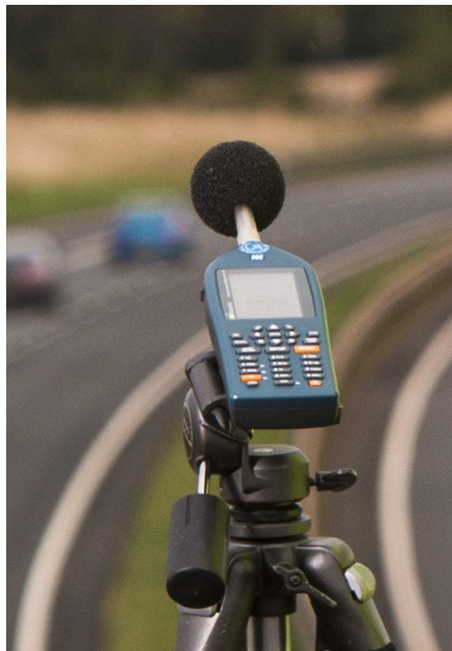
Capturing baseline noise measurements at a construction site near a motorway to determine the baseline dB level before work begins
